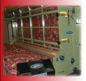
The Garnett Controls volumetric chute feed can be retrofitted to existing mechanical hoppers in order to provide increased production capabilities with uniform fibre presentation.
