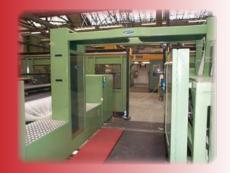
Drive chains have been replaced by 'Torque Drive Plus' Timing belts, which maintain an exact length and tension and positive carriage drive, thus minimising maintenance.
